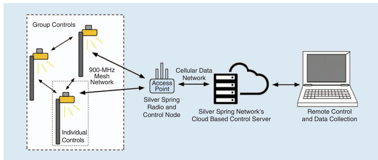
Figure 17. A configuration of a smart streetlight.
