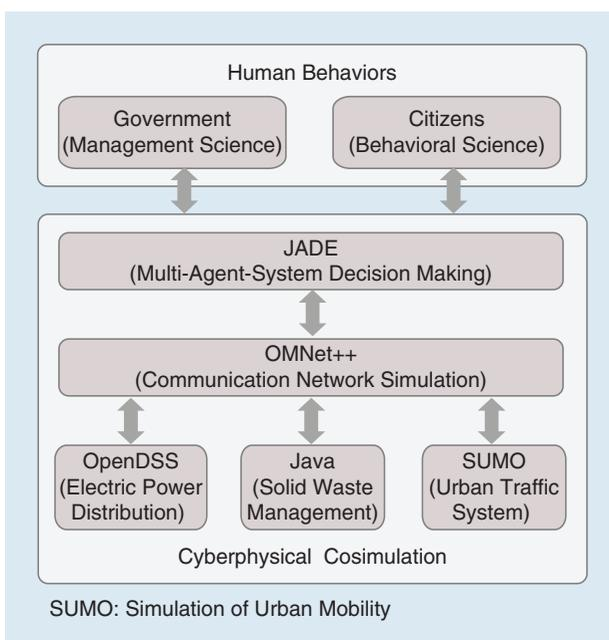
Figure 20. An MAS-based simulation platform for smart cities.
