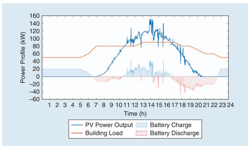
**Figure 13.** The power generation and consumption of the Keating nanogrid.
