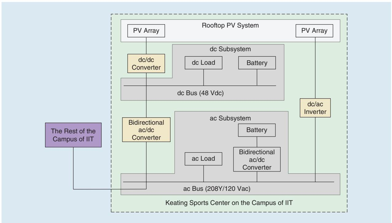
**Figure 12.** A configuration of the Keating nanogrid.
