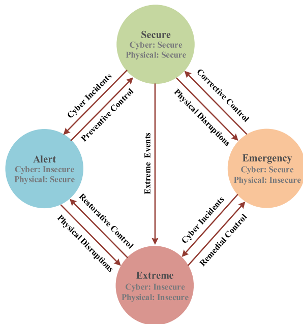
Fig. 3. Characterization of microgrid operating conditions.
